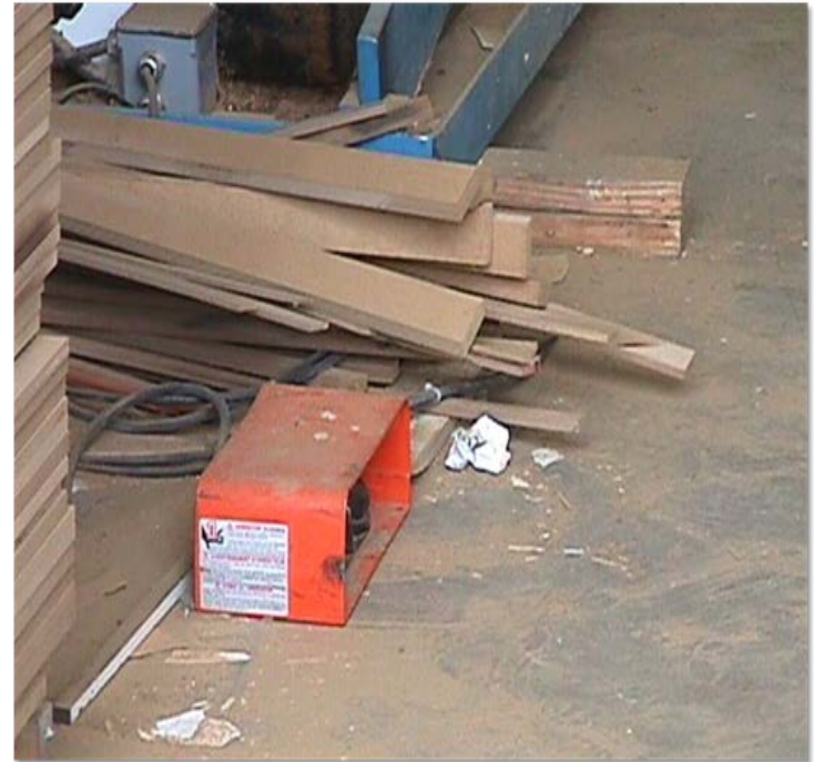
Poor housekeeping can cause trips.
